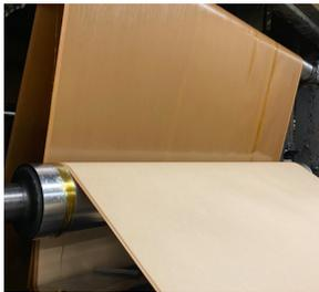
Layers of kraft paper are coated in phenolic resin and a decorative layer is added.
